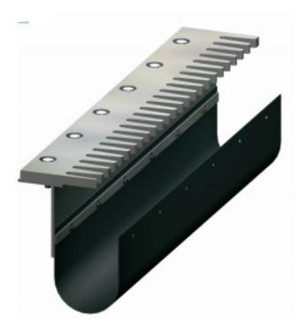
The D.S. Brown Drainage Trough System is a flexible water drainage system designed for use with open dam expansion joint systems. The D.S. Brown Drainage Trough System acts as part of the bridge drainage system by collecting runoff and channeling it into rigid downspouts, thus protecting the steel structure below from corrosion, waterways from pollution, and/or traffic from falling aggregate and roadway runoff.
