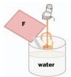
For mixing of single bags, it is acceptable to use a 25 litre steel pail as a mixing vessel, and mixing carried out using a slow speed electric drill (350/600rpm) fitted with
